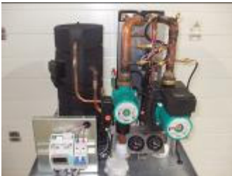
Heat pump internals
