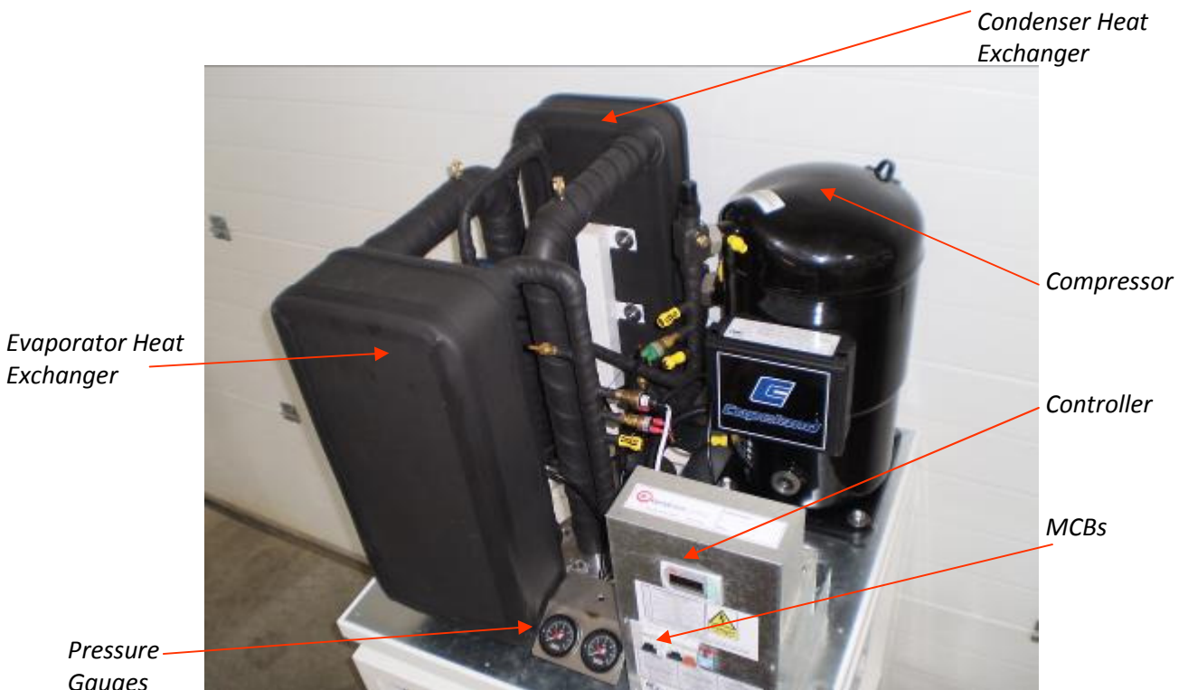
Fig 1. The internals of a heat pump
