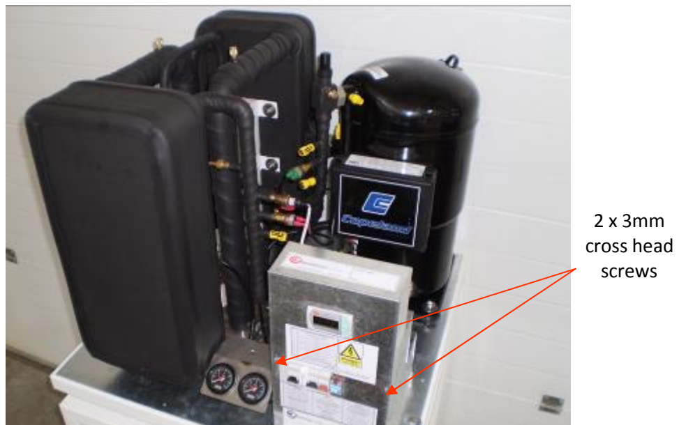
Fig 9 Position of hex screws on the electronics cover plate
